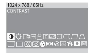
**2** Press the  $\bigtriangledown$  or  $\triangle$  buttons to highlight an OSD menu option to adjust (for example Contrast), then press the **MENU** button to select the option. The change menu for that option is displayed.
